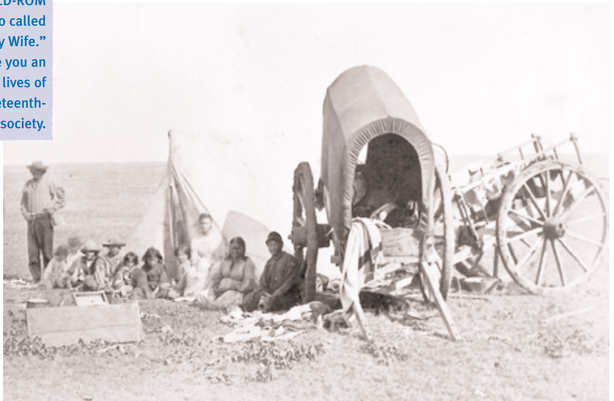
Figure 8.7 The Métis invented a unique form of transportation called the Red River cart to haul buffalo meat. These carts had large wooden wheels that were wrapped in buffalo hide. The cart was also used as a boat. The wheels were removed and hooked to the bottom. Why do you think it became the most dependable form of transportation in the Canadian West?
